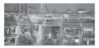
Since 2000 the historical color orthoimages have been produced from multipurpose flight color aerial images, the images were taken with a middle image scale of 1:15 000 and a focal length of 21 respectively 30 cm. The ground sampling distance of these orthoimages amounts to 25 cm.
