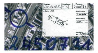
The aerial image archive of the BEV contains not only the original images but also the necessary basis for the photogrammetric applications.
