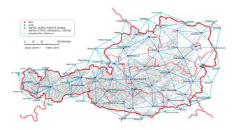
For the area covered by APOS we provide station raw data for post processing applications (APOS-PP and APOS-RAW) as well as individual correction parameter for satellite orbits, satellite clocks, ionosphere and troposphere which are computed in real time (APOS Real Time) in the form of a "Virtual Reference Station" (VRS). This correction service is offered in two accuracies:
